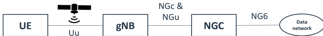
Figure 4.7-1: NTN featuring an access network serving UEs and based on a satellite/aerial with bent pipe payload and gNB on the ground (Satellite hub or gateway level)
