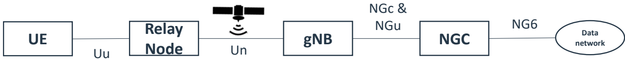
Figure 4.7-3: NTN featuring an access network serving Relay Nodes and based on a satellite/aerial with bent pipe payload
