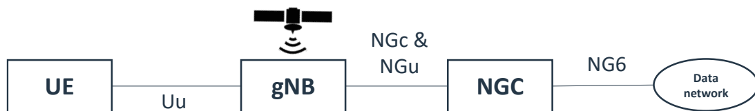
Figure 4.7-2: NTN featuring an access network serving UEs and based on a satellite/aerial with gNB on board
